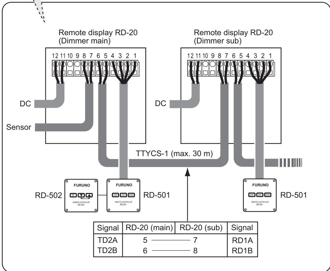
**Pattern 2: Dimmer controller is commonly used. A total of 10 RD-20s can be connected in a daisy chain. A maximum of nine sub RD-20s can be connected.**
