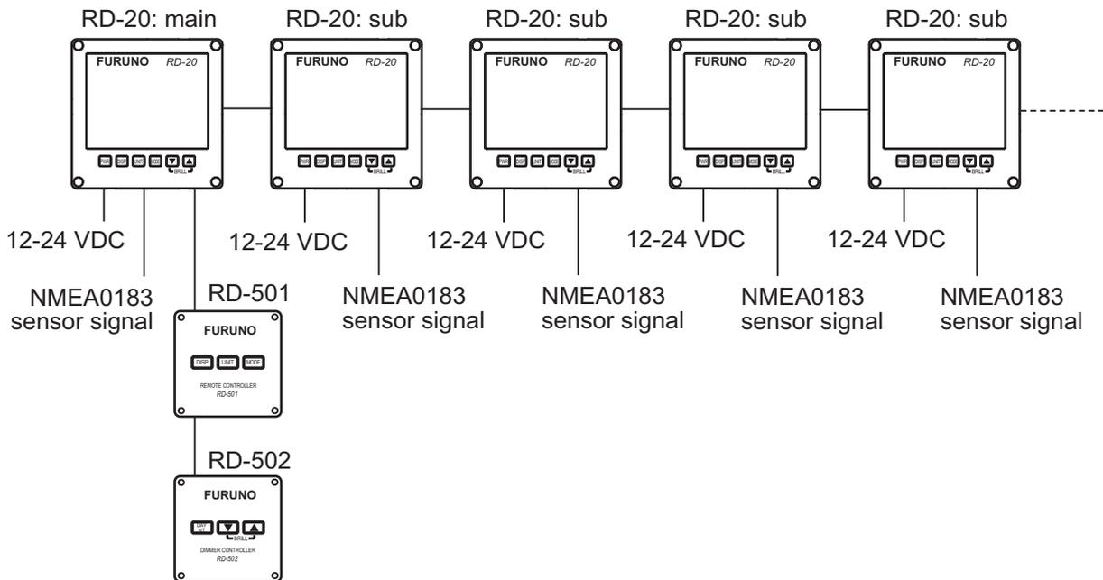
**Note:** When turning off the power for a RD-20 in the daisy chain connection, the RD-20s which are connected after that RD-20 can receive neither the sensor signal nor the brilliance signal.
