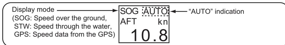
SOG/STW: The speed data from the doppler sonar, doppler log, speed log, etc. GPS: The data from the navigation equipment not described above (mainly, SOG data from a GPS navigator).
