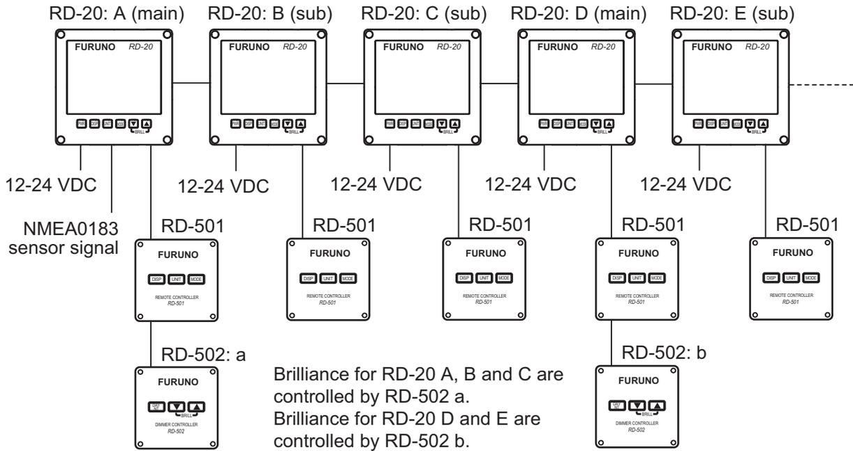
**Pattern 2: Dimmer controller is commonly used. A total of 10 RD-20s can be connected.**
