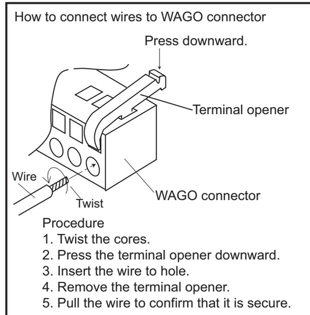
Attach the WAGO connectors (with cables). Bind the sheaths of cables to the fixture with the cable ties.
