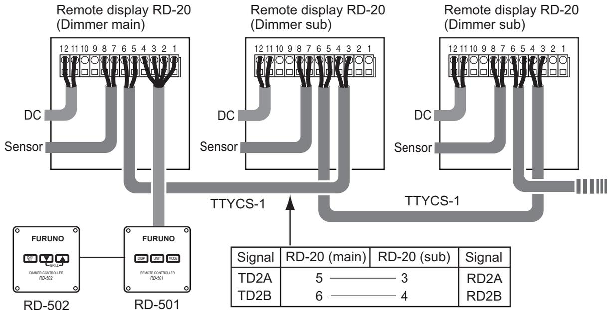
**Note:** When you turn off the power for a RD-20 in the daisy chain connection, the RD-20s which are connected after that RD-20 can receive neither the sensor signal nor the brilliance signal.
